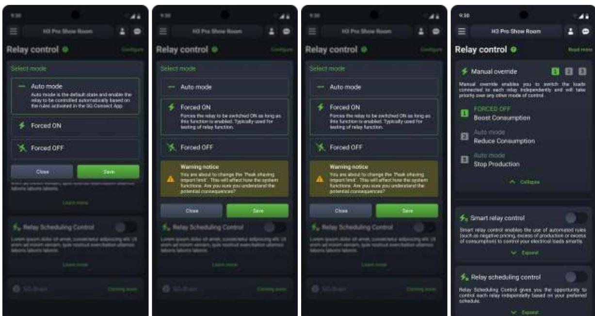
**Note:** If you activate the Manual Override function on one of the three relays, please remember to switch it back to “Auto Mode” after testing. Leaving Manual Override permanently active may quickly lead to significantly higher electricity costs (e.g., due to the continuous operation of an electric heater).
